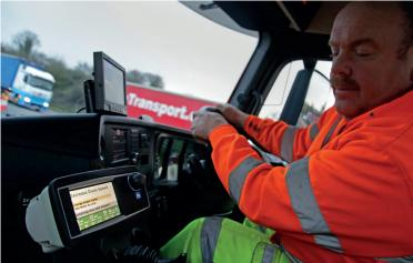
Improving safety was a key focus and the trucks are fitted with 360 degree FORS safety standard accredited cameras that aside from recoding onto a truck based hard drive also allow remote monitoring.
